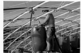
6.20 Water barrels representing partial snow load
